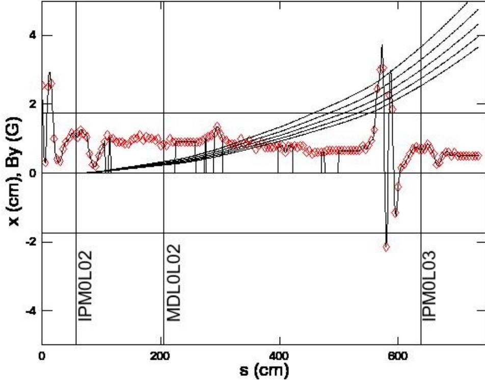
Fig. 3. Stray magnetic field measurements (red diamonds) and spline fit are used to generate  $B_y(s)$  spanning IPM0L02 to IPM0L03. The field is forced to zero for regions where mu-metal shielding is added to the beam pipe. The horizontal trajectory is plotted vs. beam position over this length for momenta (4.5, 5.0, 5.5, 6.0, 6.5 MeV/c) with initial conditions IPM0L02 ( $x=0\text{ cm}$ ,  $x'=0\text{ mrad}$ ).
