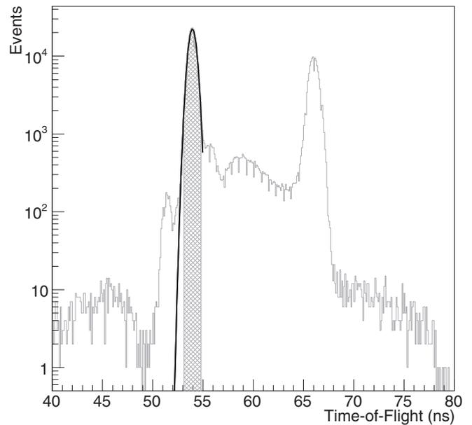
FIG. 9. A typical time-of-flight distribution of Mott coincidence triggers. Mott events from the scattering foil appear at  $\approx 54$  ns, while electrons backscattered from the beam dump are detected at  $\approx 66$  ns. Data from run 1 with the 355-nm foil.
