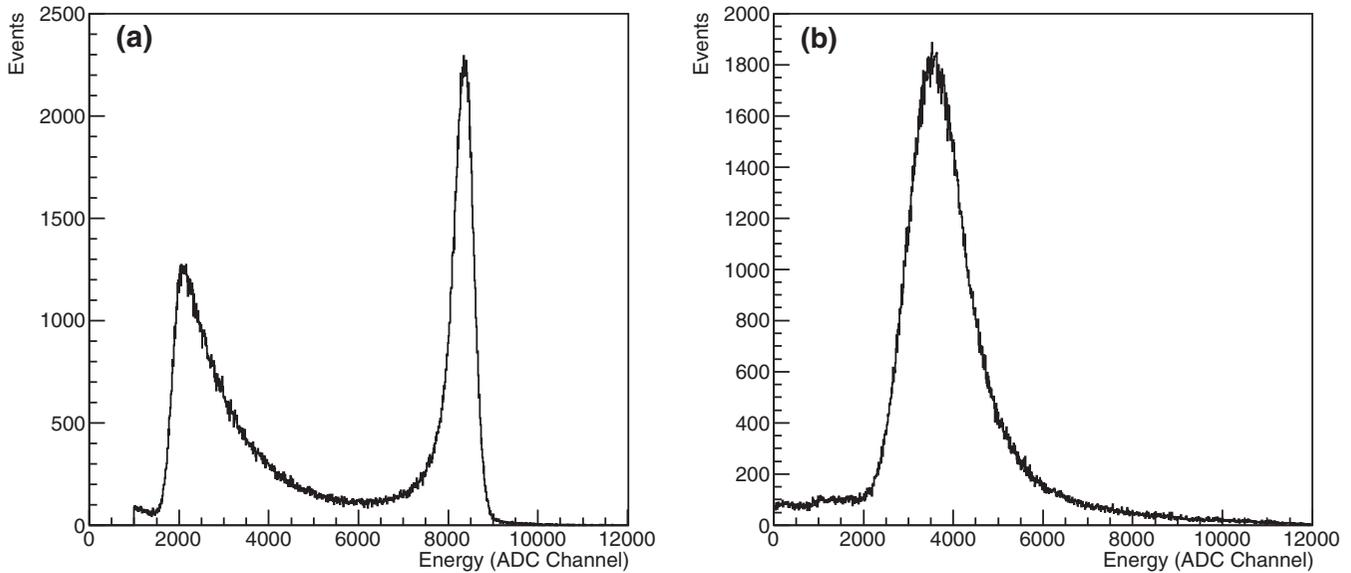
FIG. 10. Typical histograms of the (a)  $E$  and (b)  $\Delta E$  detectors. The  $E$  threshold was set to  $-25$  mV for these data and no timing cut was applied. Data from run 1 with the 355-nm foil.
