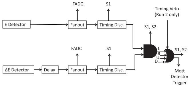
FIG. 8. Electronic signal processing of the  $\Delta E$  and  $E$  signals (the “left” of four detector arms).
