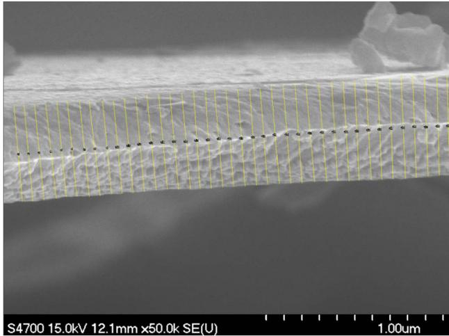
FIG. 23. FESEM image of a nominal 625-nm-thick gold foil mounted on a silicon substrate (lower dark region). Many measurements of the thickness along this region indicate the foil is  $561.2 \pm 31.0$  nm. Yellow lines with black labels denote the lines used for thickness analysis with ImageJ software [62].
