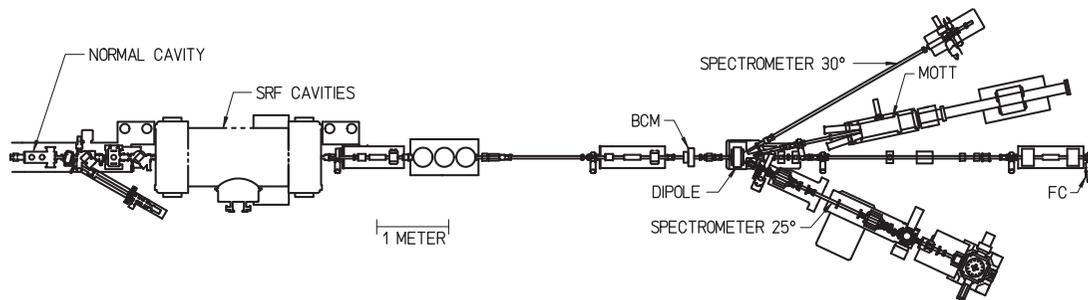
FIG. 4. Plan view of the injector illustrating the rf accelerating cavities, the 12.5° beam line through the Mott polarimeter, the spectrometer beam lines at  $-30^\circ$  and  $25^\circ$ , and the straight beam line leading to the rest of the CEBAF injector including an rf cavity beam current monitor (BCM) and a Faraday cup (FC).
