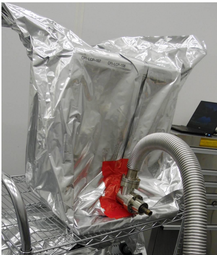
Figure 4.1: Pumping line installed on RAV
