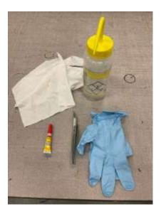
Once the surface is clean you will apply several small drops of super glue (non-gel) to the surface. Do not completely cover the surface with super glue, a few drops on the corners and along the center will hold the indium in place while the part is installed. (as seen in the image below)
