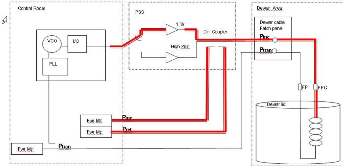
**Figure A11.** Block diagram representation of 'Forward Power to detuned cavity' cable calibration step.
