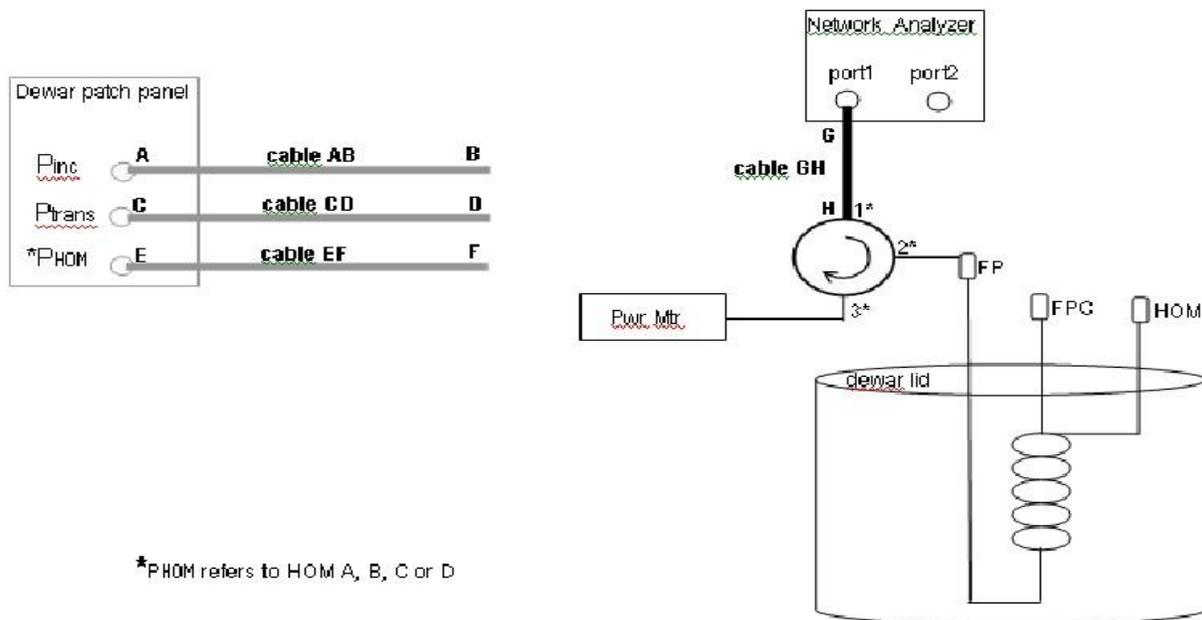
**Figure A8.** Cable GH, cavity field probe (FP) and power meter connected to circulator for ‘Transmitted Cable Return Loss’ field probe measurement. The same measurement is made for each HOM if instrumented.
