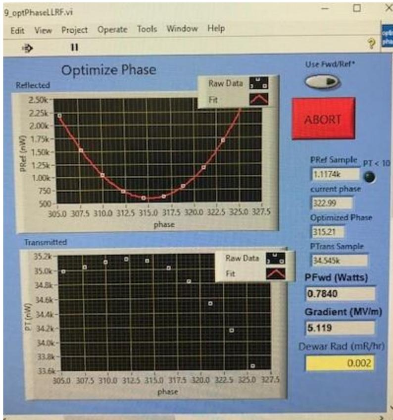
**Figure 3.** A well phased cavity will have a similar shape as shown in the graphs.
