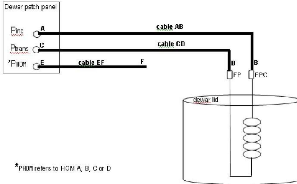
**Figure A10.** Cable AB to Fundamental Power Coupler (FPC) port and Cable CD to Field Probe (FP) port for 'Incident power to detuned cavity' cable calibration step.
