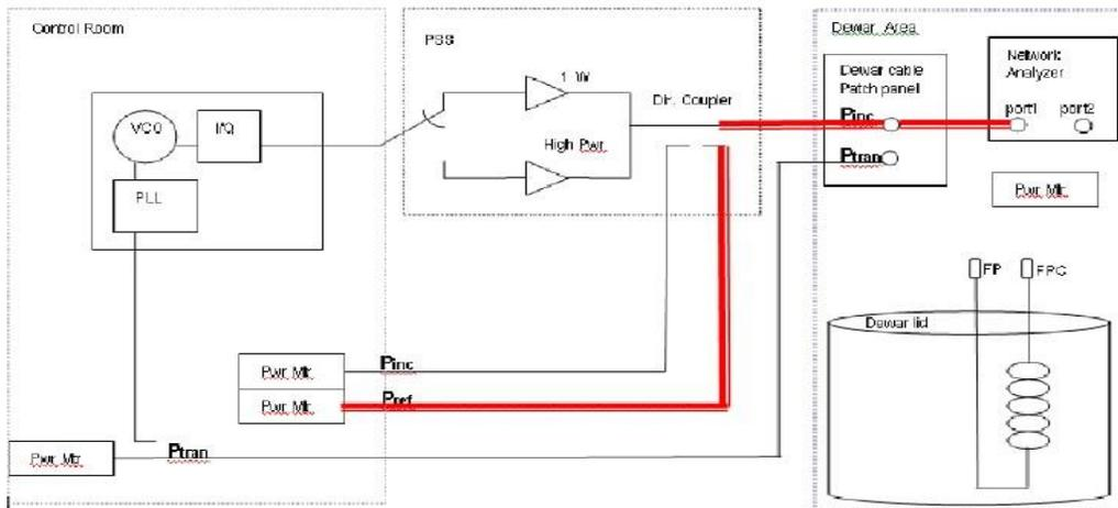
**Figure A2.** Block diagram representation of ‘reflected power from VTA’ cable calibration step.
