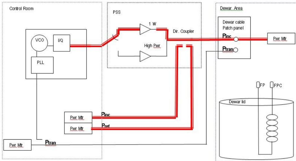
**Figure A4.** Block diagram representation of ‘incident power measured at dewar’ cable calibration step.
