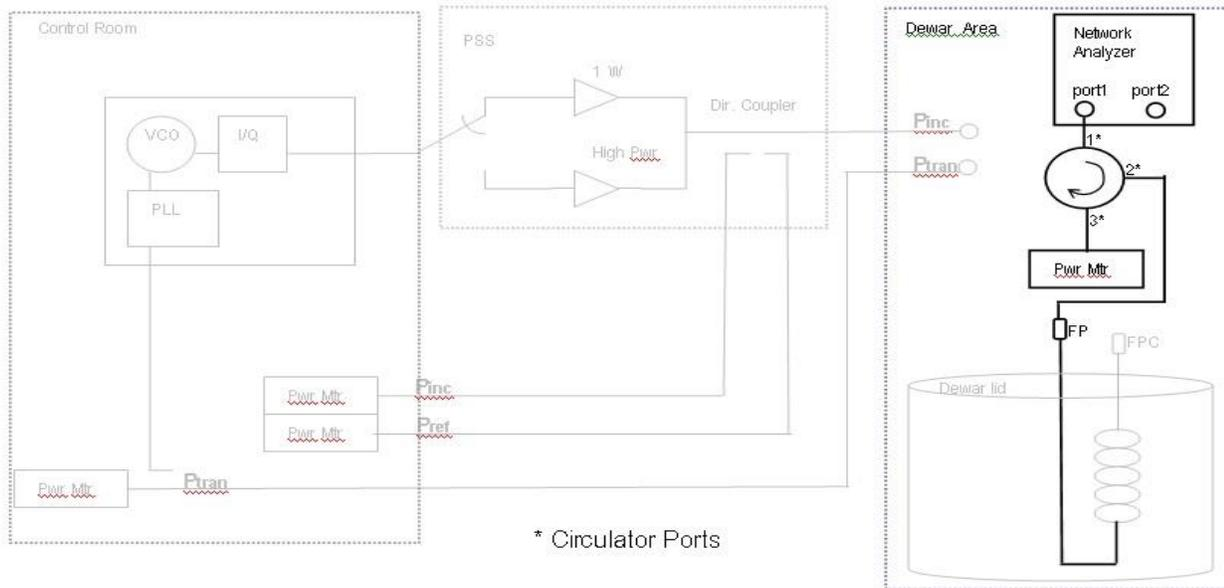
**Figure A9.** Block diagram representation of ‘transmitted cable return loss’ field probe cable calibration step.
