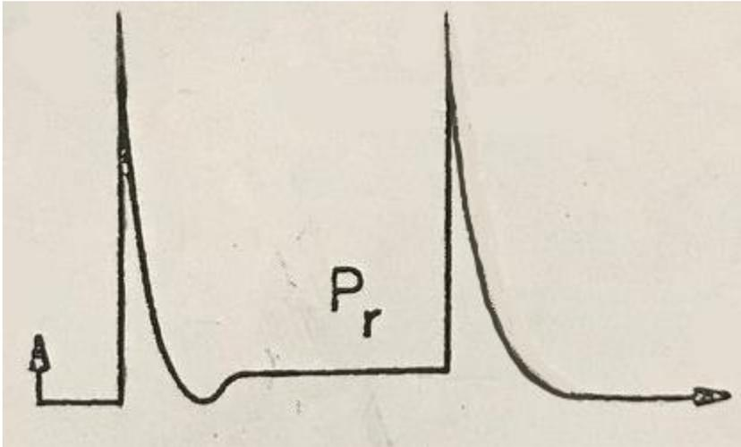
**Figure 5.** A cavity that is critically coupled will have a transition on the reflected power where it transitions towards 0W and recovers at a slightly higher value. Undercoupled cavities do not have this transition.
