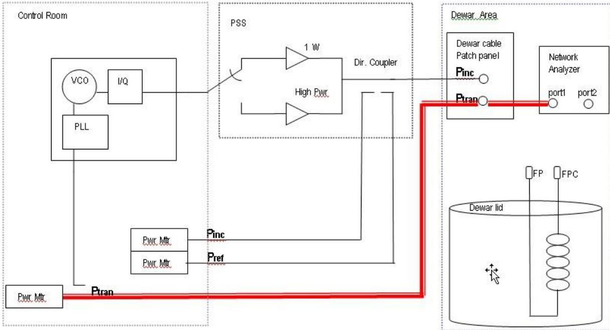
**Figure A6.** Block diagram representation of ‘transmitted power to control room’ cable calibration step.
