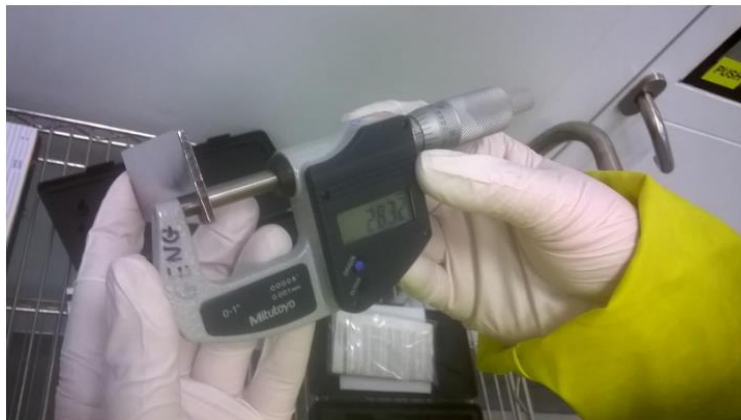
Figure 1: measurement of the thickness of the Nb sample with a digital micrometer at a fixed, marked location
