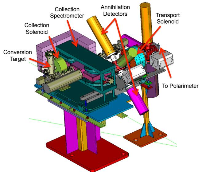
Figure 1: The main components of the PEPPO positron production, collection and detection.
