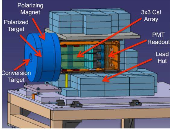
Figure 2: The main components of the PEPPo Compton transmission polarimeter.
