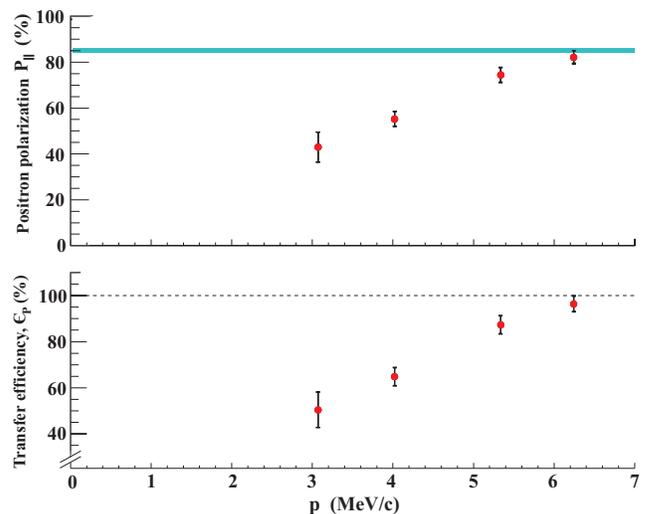
FIG. 3. (Color) PEPPo measurements of the positron polarization (top panel) and polarization transfer efficiency (bottom panel); statistics and systematics are reported for each point, and the shaded area indicates the electron beam polarization.
