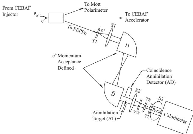
FIG. 1. Schematic of the PEPPo line and apparatus illustrating the principle of operation of the experiment based on the processes sequence  $e^- \xrightarrow{T1} \gamma \xrightarrow{T1} e^+ \xrightarrow{T2} \gamma \xrightarrow{S3} \gamma$  described in the text. The setup footprint is about  $3 \times 1.5 \text{ m}^2$ .
