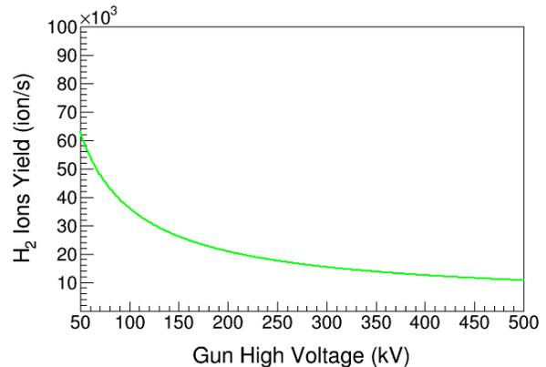
FIG. 6. (Color) Ions yield assuming electron beam current of 2.0 mA and gun vacuum of  $8.0 \times 10^{-12}$  Torr.
