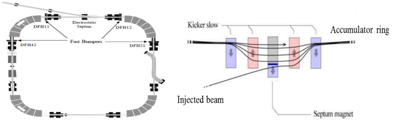
FIG. 7. (Color) Low Energy Ion Ring (LEIR) at CERN (left) and LEIR injection magnets (right).
