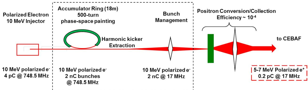
FIG. 4. (Color) 10 MeV polarized electron injector provides bunches that are accumulated 500 turns in an accumulator ring before being extracted to a positron conversion target, where polarized positrons are created and collected to a beam of about 5 MeV.
