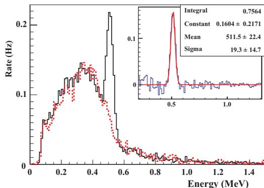
FIG. 2. (Color) Measured energy spectra in one of the annihilation detectors (AD) once T1 is inserted in (full line) or removed from (dash line) the electron beam path; the top right corner shows the difference between these spectra.
