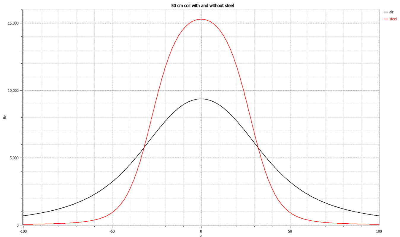
Figure 10. B_z(0,0,z) of 50 cm long, 60 cm ID, 108 cm OD coil, with (red) and without (black) steel.
