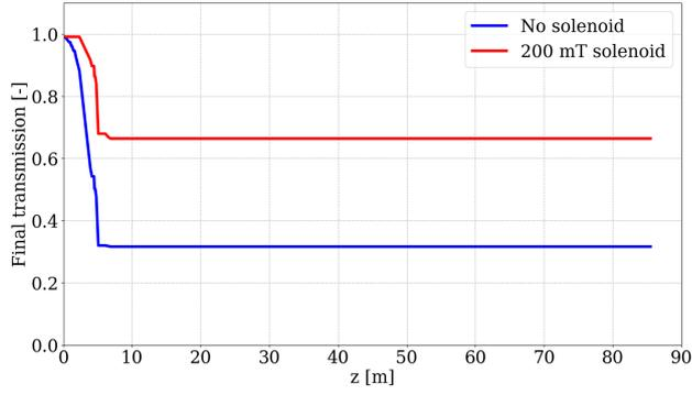
Figure 3: Simulated transmission comparison between runs without and with a 200 mT solenoid downstream of the second aperture. Target thickness for this run is 1  $\mu\text{m}$  and the collimators aperture holes radius are 3 mm and 8 mm.
