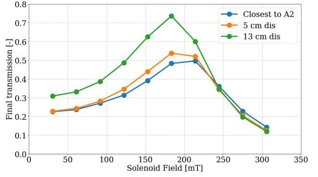
Figure 4: Simulated transmission at the end of the CEBAF injector chicane for different Solenoid field values and longitudinal displacement from the closest position to the second collimator. These simulations were done with a 1  $\mu\text{m}$  thick target and collimator aperture holes of 3 mm and 6 mm radius.
