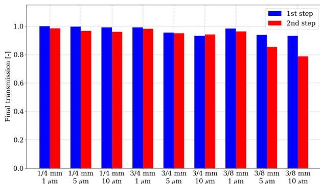
Figure 6: Optimized transmission from the end of the degrader to the end of the CEBAF injector chicane. Optimizations were performed for three different target thicknesses ( $1 \mu\text{m}$ ,  $5 \mu\text{m}$ ,  $10 \mu\text{m}$ ) and three collimator aperture hole size combinations ( $1 \text{ mm}/4 \text{ mm}$ ,  $3 \text{ mm}/4 \text{ mm}$ ,  $3 \text{ mm}/8 \text{ mm}$ ).
