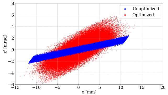
Figure 7: Horizontal phase space comparison between optimized and unoptimized runs. Target thickness for this run is  $1 \mu\text{m}$  and the collimators aperture holes radius are  $3 \text{ mm}$  and  $8 \text{ mm}$ .
