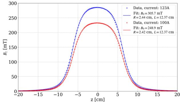
Figure 5: Fitted functions to measured Solenoid magnetic field map. Measurements were fitted to equations (1) via the  $B_0$ ,  $L$  and  $R$  parameters.
