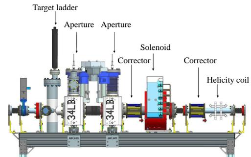
Figure 2: Model of the electron beam degrader.
