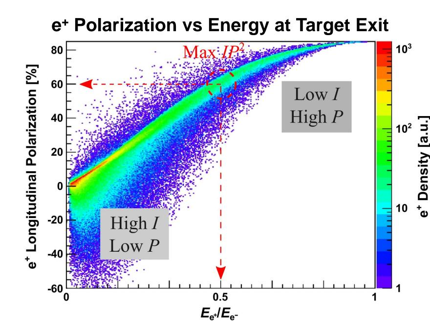
For max Figure-of-Merit ( $FoM = IP^2$ , where is  $e^+$  current and P is  $e^+$  polarization):
