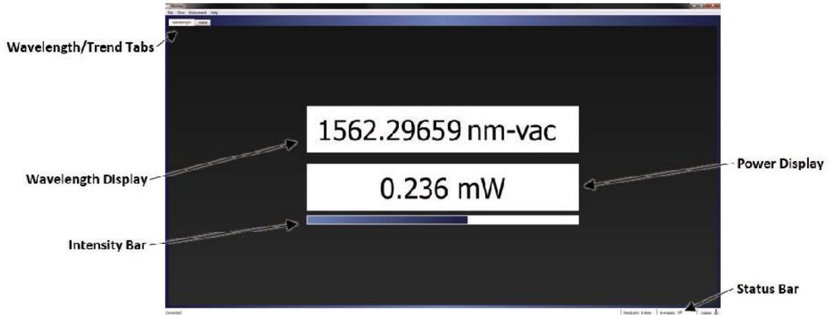
**Figure 5.2: Wavelength Screen of VIS and NIR Versions**
