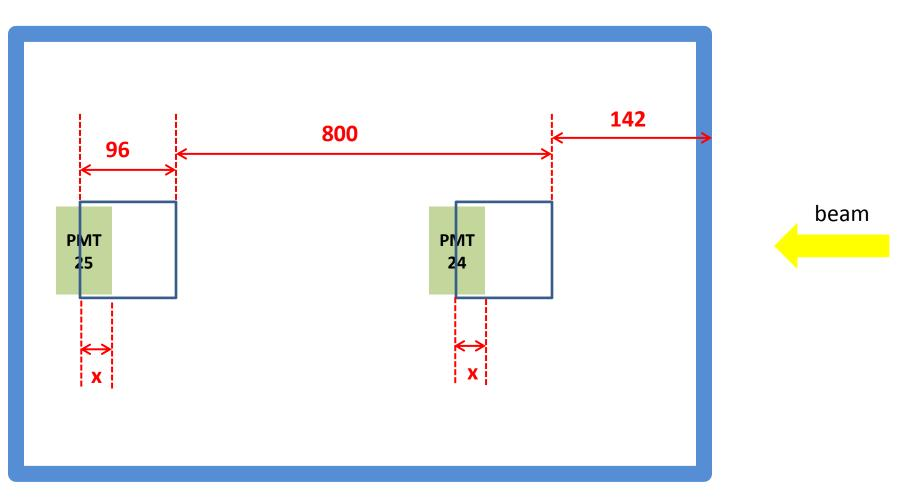
x=distance between thePMT entrance window and the edge of the support, it depends on how the PMT was placed
