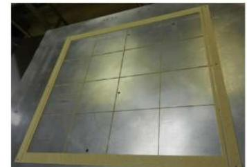
Support frame for GEM with 300  $\mu\text{m}$  spacers inside the active area
