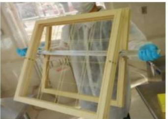
Frames on a custom holder for cleaning in Ultrasonic bath
