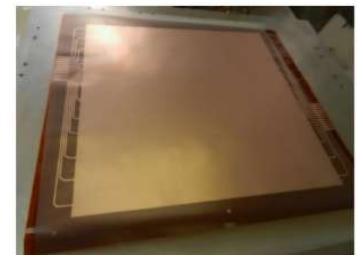
GEM foil with the visible contact of the HV sectors
