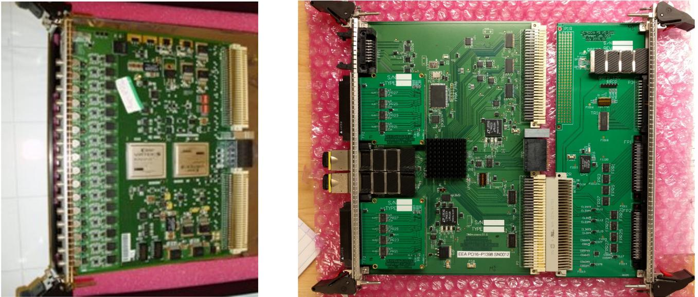
FIG. 33. Left: FADC250 - JLab 16 channel VME/VXS based 250MSPS Flash ADC digitizer. Right: VETROC - JLab 128 channel TDC. Expansion/rear transition card that supports an additional 64 TDC channels is shown.
