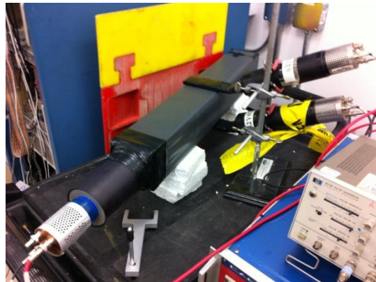
Figure 5 Prototype setup for testing the best optical contact in SHMS preshower.
