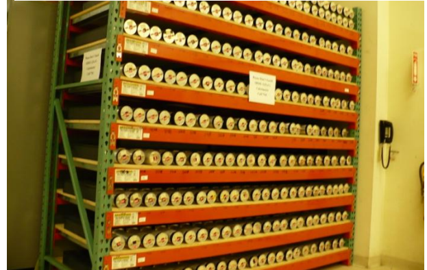
Figure 3 The refurbished HERMES lead glass that is ready to be installed in the SHMS.
