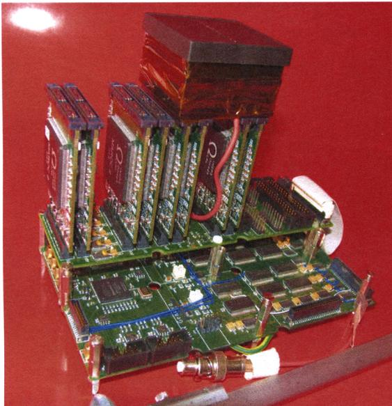
Fig. 5. Picture of the system prototype. Note that the CB and the BP are arranged in order to minimize space occupancy.
