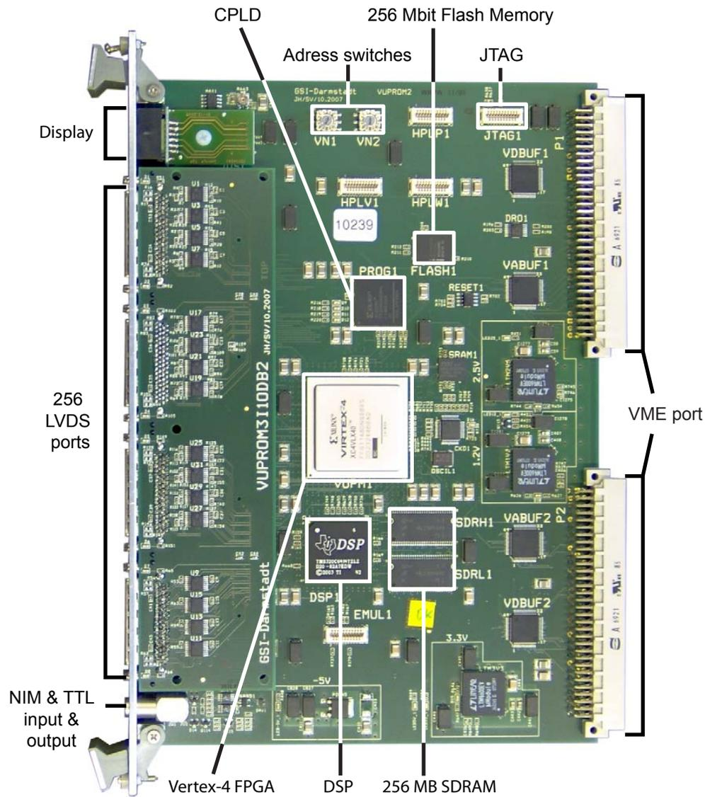
**Figure 2.16:** Photograph of the logic module VUPROM used in the trigger system of the fiber detector. The LVDS ports, at left, are divided in 8 individual ports handling 32 channels each, making a total of 256.
