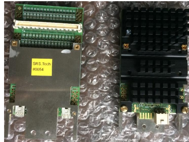
SRS-VMM3 with cooling structure
