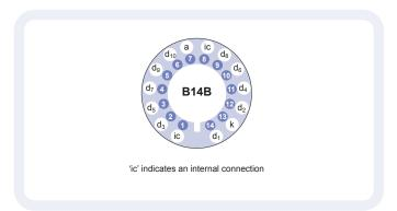
Our range of B14B sockets is available to suit the B14B hardpin base. The socket range includes versions with or without a mounting flange, and versions with contacts for mounting directly onto printed circuit boards.
