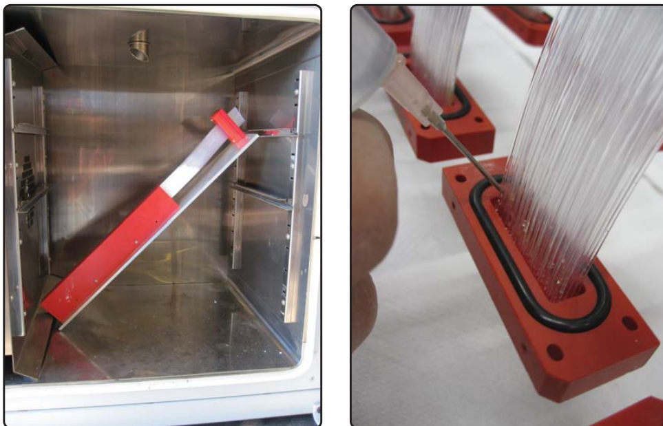
Figure 2.36: Left. Photography of the aluminium plate with the bundle into the air flow oven. The size of the oven allows to place three plates at time. Right. Detail of the application of the glue into the cookie with a syringe. The cookie has an O-ring placed.
