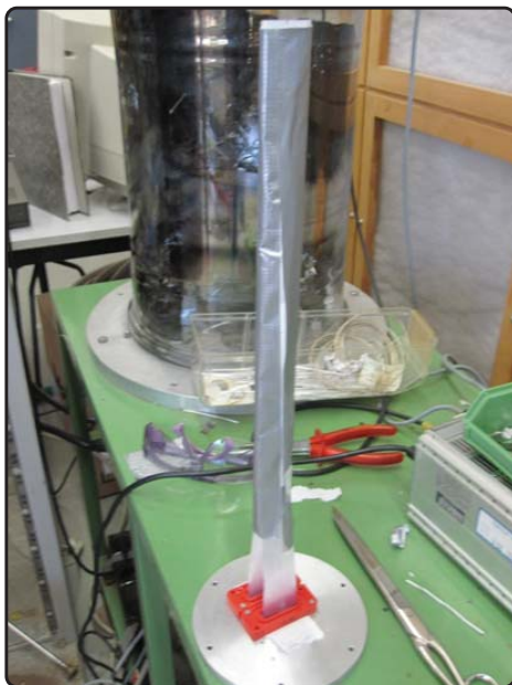
(a) Photography of two bundles attached to the cap covered and ready for aluminization.
