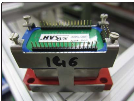
Figure 2.39: Left. Photography of the cookie with the aluminium clamping plates. Right. Detail of the fasten screws at bottom of the PMT base.
