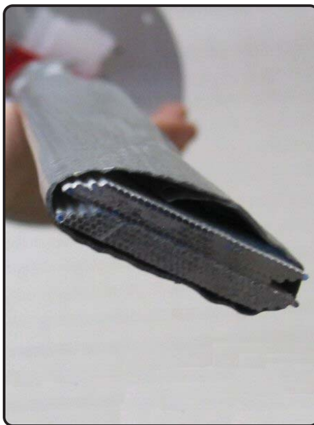
(b) Photography of the two bundles after the aluminization..
