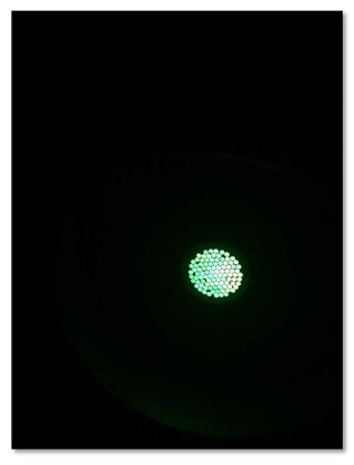
We wrap the bottom of the prototype in black paper and turn off all light. Then we use a glim to shine the bottome of prototype. We can see that every fiber is bright, so we confirm that no fiber is broken when inserting.
