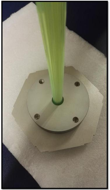
We glued the fiber into the hole with spoxy resin and these fibers had been cut by Kedi.
