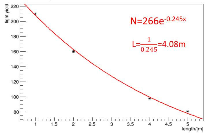
By using  $N=N_0 e^{lx}$  and  $L=\frac{1}{l}$ , we can get the clear fiber attenuation length:  $N=266e^{-0.245x}$
