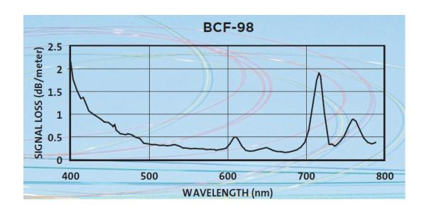
dB = 10 \* log N, N is attenuation ratio. For clear fiber with 495 nm wavelength, the dB/m is -0.5, which equal to the N = 0.89.  $(0.89)^x = 1/e$ , x=8.68m. (amplitude??)
